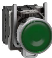
Illuminated push button, metal, flush, green, Ø22, spring return, 230...240 V AC, 1 NO + 1 NC
