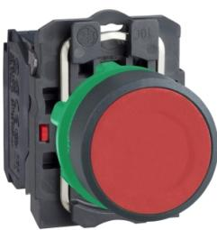
Push button, plastic, flush, red, Ø22, spring return, unmarked, 1 NC
