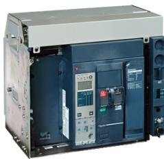
Circuit breaker frame, MasterPact NT06H1, 630A, 42kA/440VAC 50/60Hz (Icu), 4 poles, drawout, without control unit
