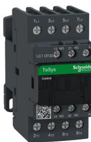
IEC contactor, TeSys Deca, nonreversing, 32A resistive, 4 pole, 4 NO, 110VAC 50/60Hz coil, open style
