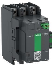
High power contactor, TeSys Giga, 3 pole (3NO), AC-3  $\leq 440\text{V}$  225A, standard version, 100...250V wide band AC/DC coil
