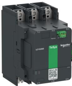
High power contactor, TeSys Giga, 3 pole (3NO), AC-3 <=440V 400A, standard version, 100...250V wide band AC/DC coil
