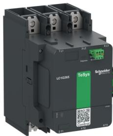
High power contactor, TeSys Giga, 3 pole (3NO), AC-3 <=440V 500A, standard version, 100...250V wide band AC/DC coil
