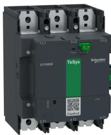
High power contactor, TeSys Giga, 3 pole (3NO), AC-3 <=440V 800A, standard version, 100...250V wide band AC/DC coil
