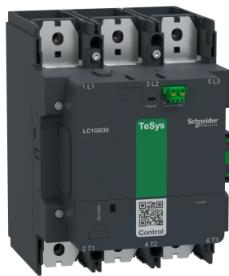
High power contactor, TeSys Giga, 3 pole (3NO), AC-3 <=440V 630A, standard version, 100...250V wide band AC/DC coil
