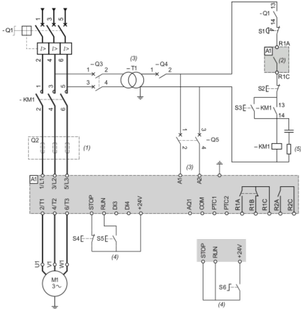
(1) : Installation of additional fast-acting fuses is mandatory to upgrade to type 2 coordination according to IEC 60947-4-2.
