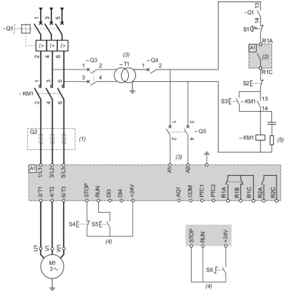
(1) : Installation of additional fast-acting fuses is mandatory to upgrade to type 2 coordination according to IEC 60947-4-2.
