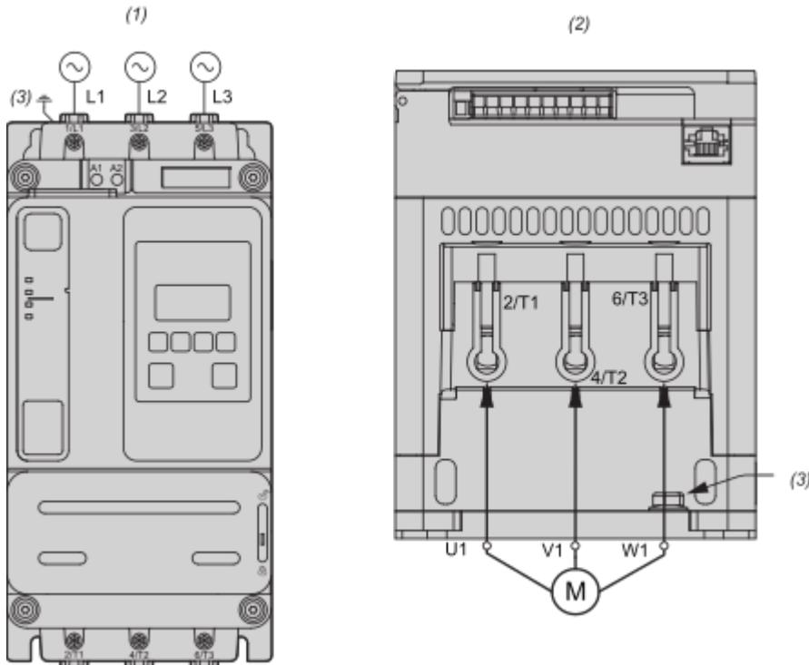
Use class C cables for the power connections.
